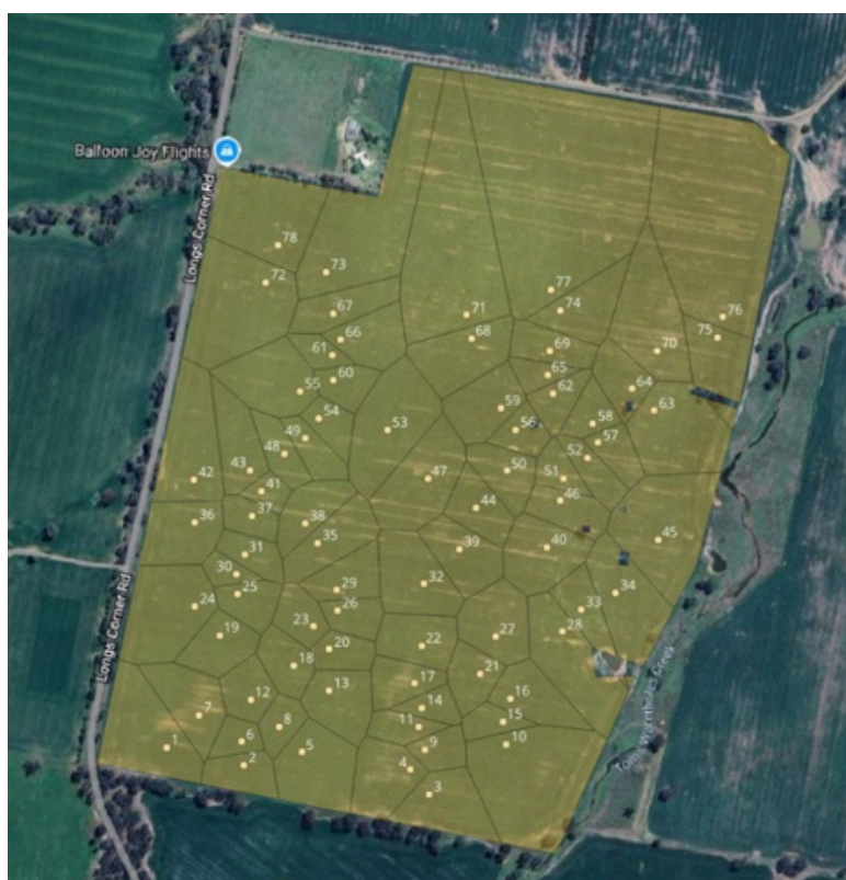
Fig. 7. Voronoi soil zone map. The paddock is split into soil zone polygons which are centred around where soil samples were taken. These zones are then used to attach additional information such as yield, and topographical data.
